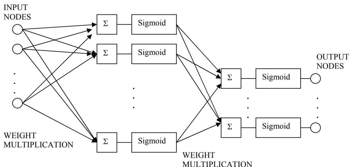
Fig. 1 Multilayer perceptron neural network model
