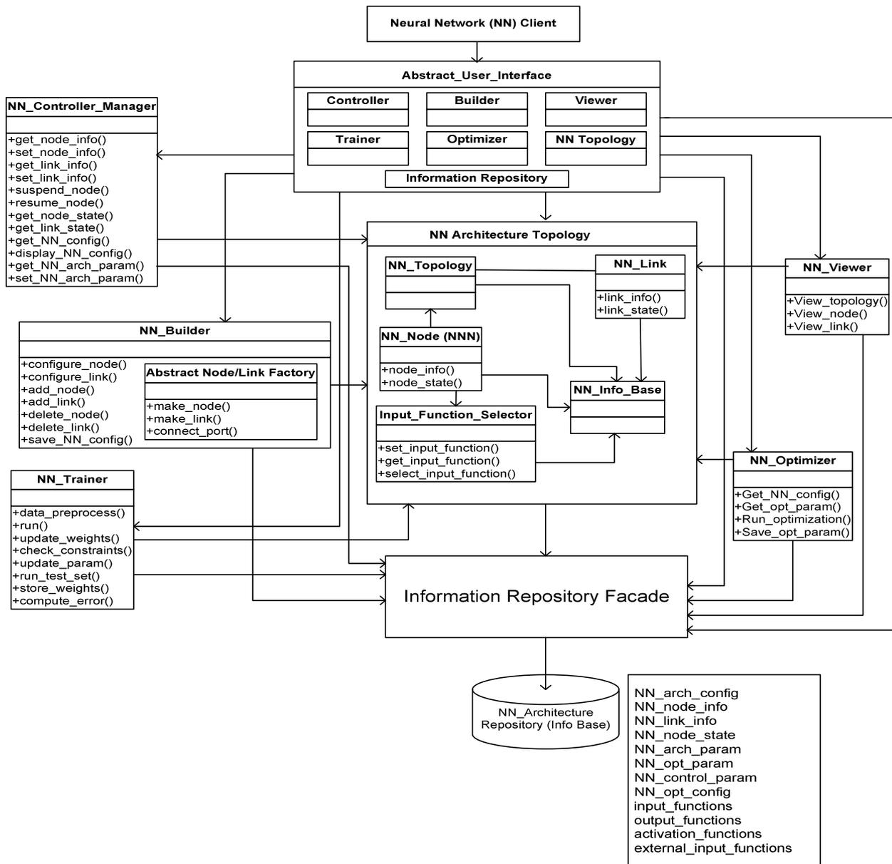
Fig. 2 Neural network software architecture information model
