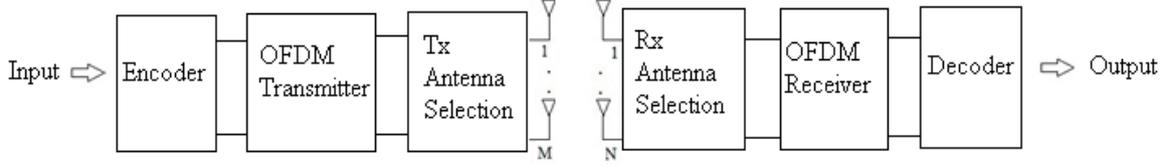
Figure 1. Coded OFDM system with antenna selection
