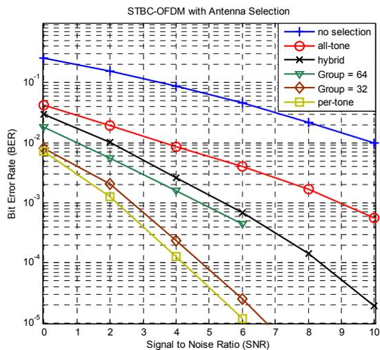
Figure 2. STBC-OFDM with Joint Transmit and Receive Antenna Selection
