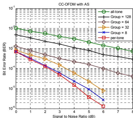
Figure 3. CC-OFDM with Joint Transmit and Receive Antenna Selection
