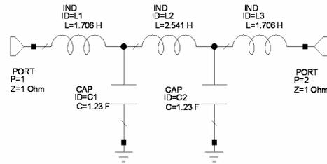
Figure 5. Lumped-element prototype filter, (normalized element values:  $L_1 = L_3 = 1.7058$ ,  $L_2 = 2.5408$ ,  $C_1 = C_2 = 1.2296$ ,  $R_G = R_L = 1$ ).
