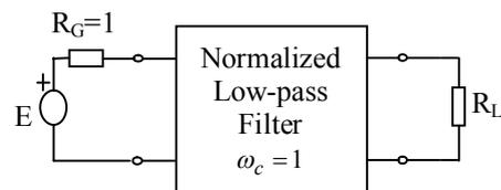
Figure 1. Normalized low-pass prototype filter with the generator impedance  $R_G=1$ , cutoff frequency  $\omega_c=1$ .
