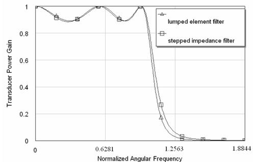
Figure 6. Transducer power gain curves of the lumped- and stepped impedance prototype filters.
