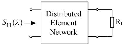
Figure 2. Darlington representation of a distributed-element network.
