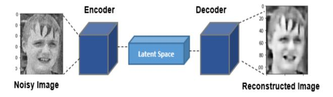
*Figure 3.* The basic representation of an autoencoder
