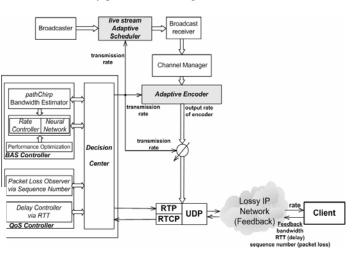
Fig. 6 BAS Controller, QoS Controller and Decision Center with Encoder and Transmitter
