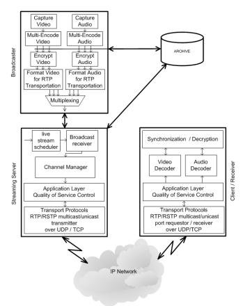
Fig. 2 Internal Structure of Video Streaming
