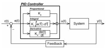
Fig. 4 General Structure of PID Controller in a control system
