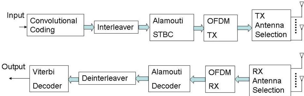
Figure 1: Block diagram of proposed STC-OFDM system with transmit and receive antenna selection
