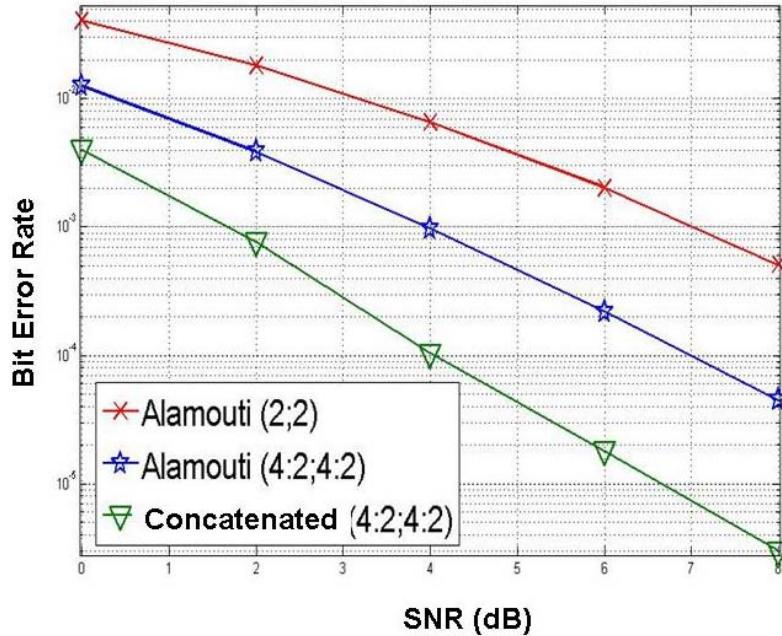
Figure 2: Bit error rates with all-tone antenna selection
