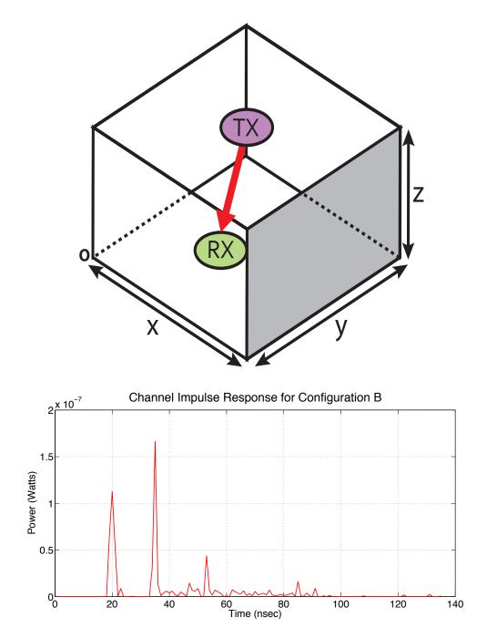
Figure 3.8. Structure and Channel Impulse Response of Configuration B
