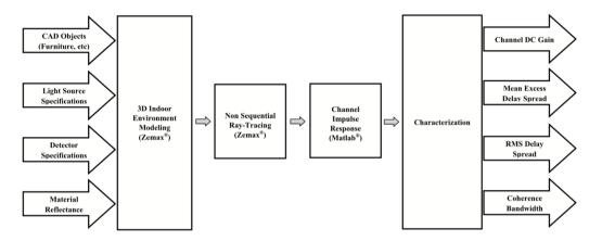
Figure 3.2. Steps of the Zemax<sup>®</sup> procedure [18]
