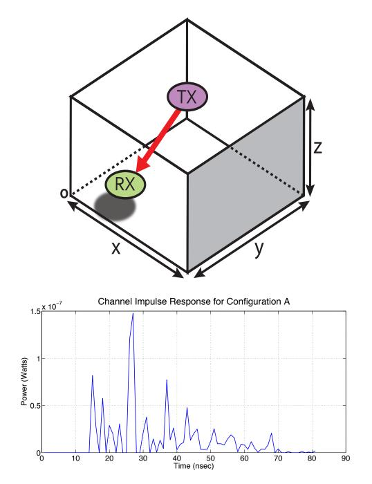
Figure 3.7. Structure and Channel Impulse Response of Configuration A
