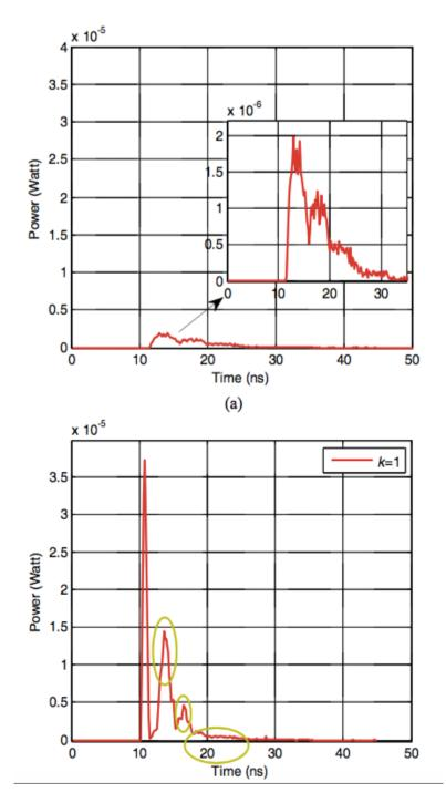
Figure 3.5. Empty room channel impulse response (with first order reflections) [18]
