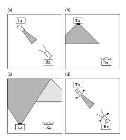
Figure 1.1. LOS Configurations [19]
