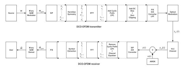
Figure 4.2. DCO Block Diagram
