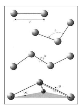
**Figure 2.2.** Bonded interactions: r shows bond stretching;  $\theta$  is the bond angle term;  $\varphi$  gives the dihedral angle; the small out-of-plane angle  $\alpha$  is governed by the so-called "improper" dihedral angle<sup>4</sup>
