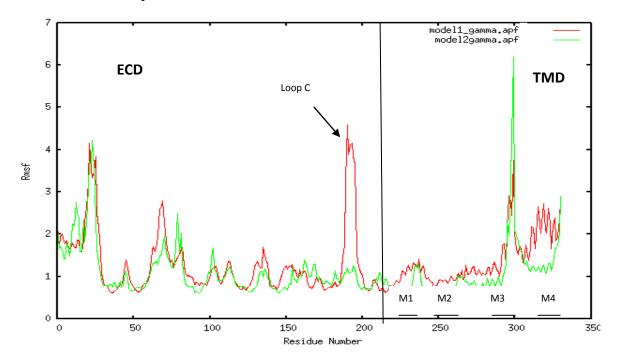
**Figure 3.6 :** Comparison of the fluctuations of C alpha atoms in two gamma subunits of two model, C Loop motions reduced.
