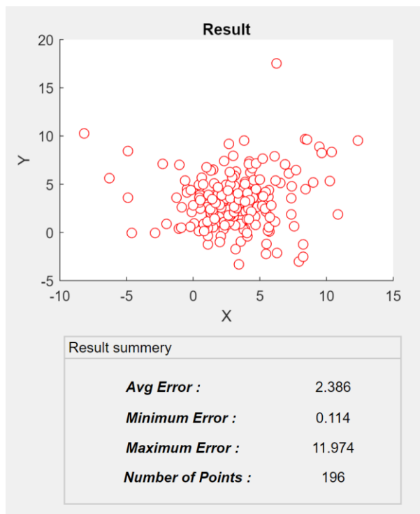
Figure 6.12: Results with est. n in 6*6 room size with 40 cm grid size, 3 dBm noise
