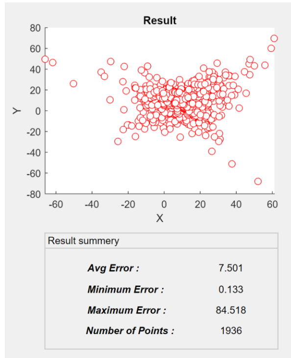
Figure 6.18: Results with est. n in 18*18 room size with 40 cm grid size, 3 dBm noise
