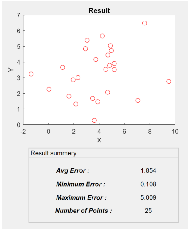
Figure 6.10: Results with est. n in 6*6 room size with 100 cm grid size, 3 dBm noise
