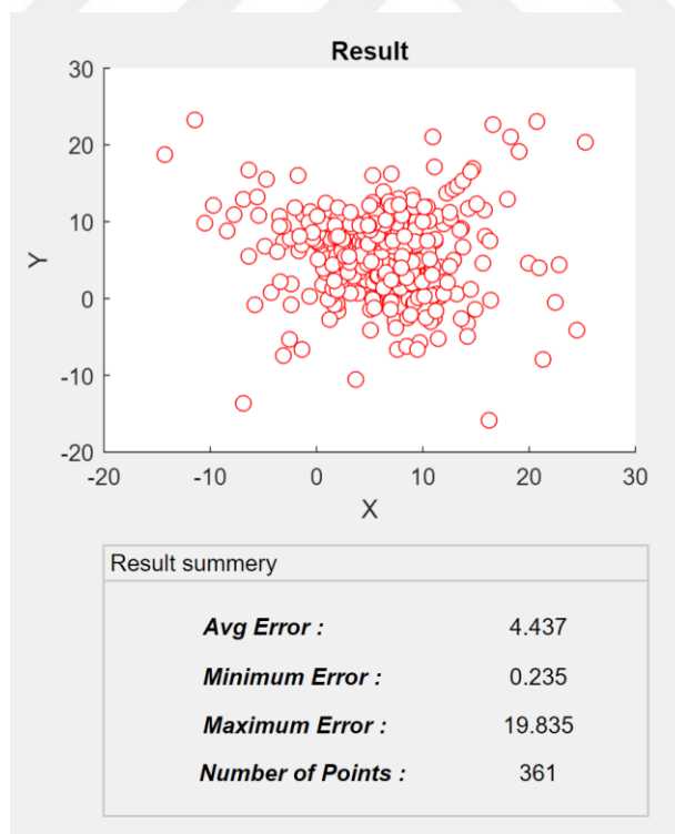
Figure 6.14: Results with est. n in 12*12 room size with 60 cm grid size, 3 dBm noise
