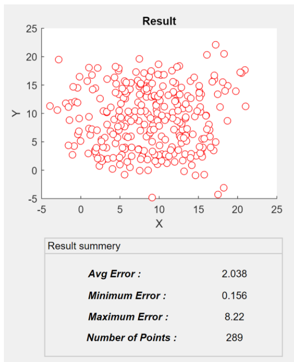
Figure 6.7: Results with est. n in 18*18 room size with 100 cm grid size, 1dBm noise
