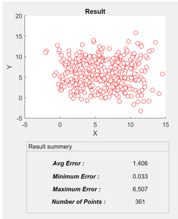
Figure 6.5: Results with est. n in 12*12 room size with 60 cm grid size, 1dBm noise
