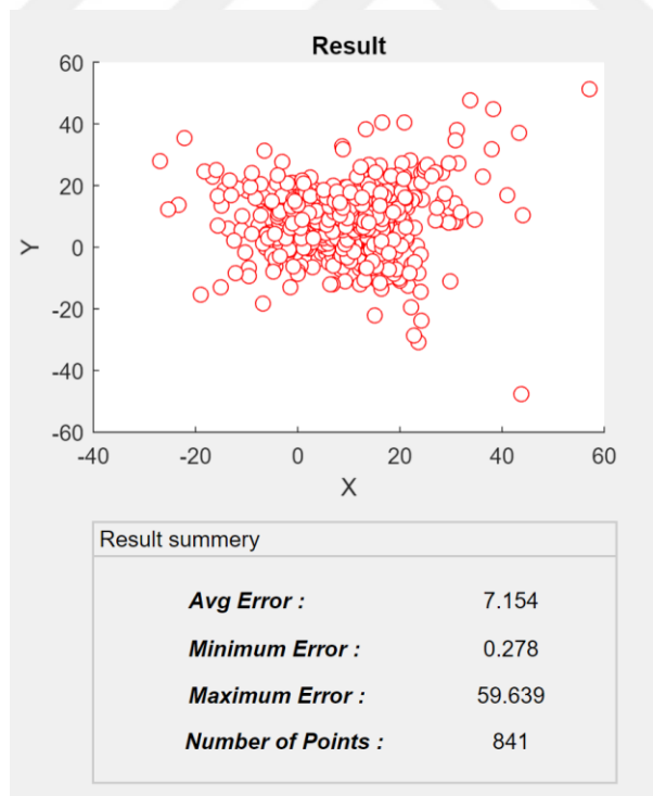
Figure 6.17: Results with est. n in 18*18 room size with 60 cm grid size, 3 dBm noise
