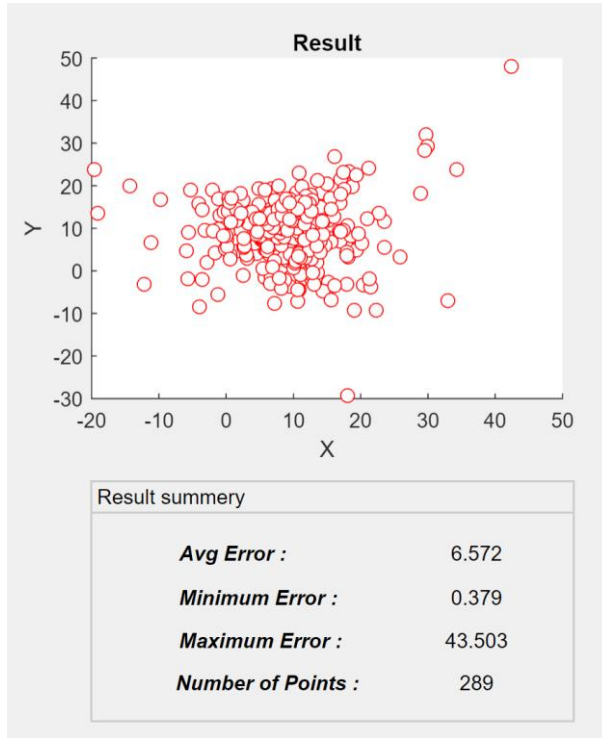
Figure 6.16: Results with est. n in 18*18 room size with 100 cm grid size, 3 dBm noise
