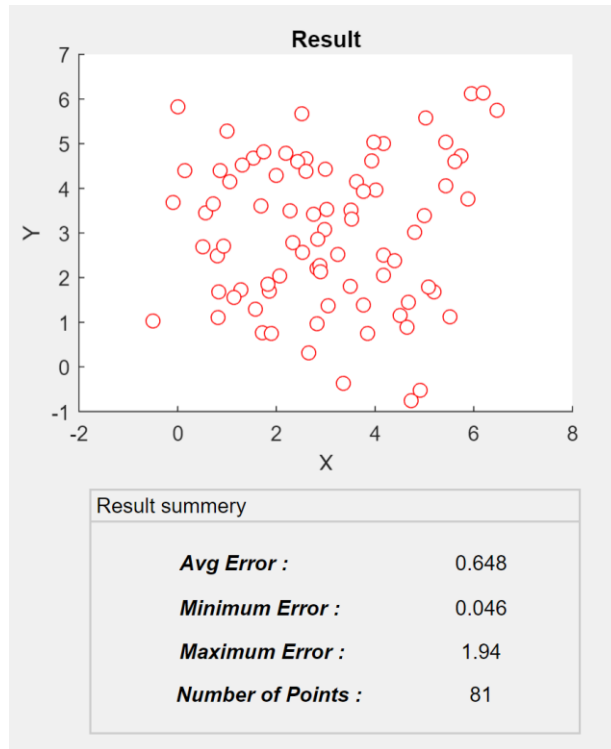
Figure 6.2: Results with est. n in 6*6 room size with 60 cm grid size, 1dBm noise
