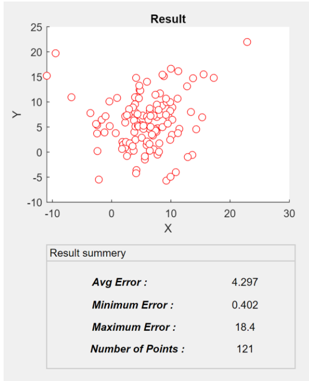
Figure 6.13: Results with est. n in 12*12 room size with 100 cm grid size, 3 dBm noise
