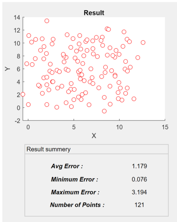
Figure 6.4: Results with est. n in 12*12 room size with 100 cm grid size, 1dBm noise
