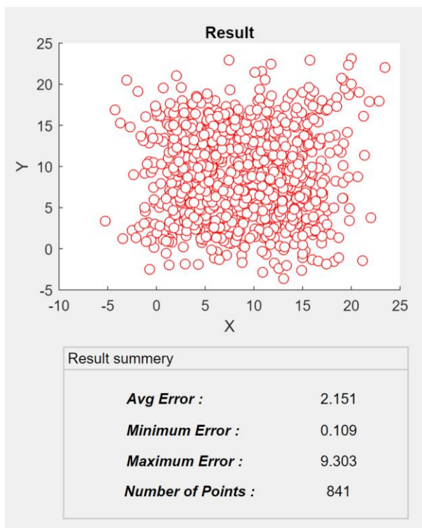
Figure 6.8: Results with est. n in 18*18 room size with 60 cm grid size, 1dBm noise
