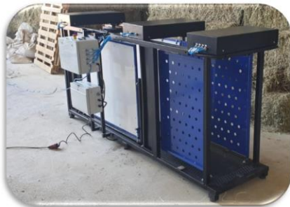
Automated counting, weighting and drafting crate
