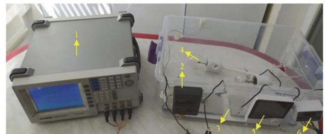
Figure 4 The designed system using four-plate horizontal capacitive coupler structure: (1) LCR meter, (2) digital thermometer, (3) horizontal coupler, (4) bulb, (5) humidity meter, (6) temperature controller
