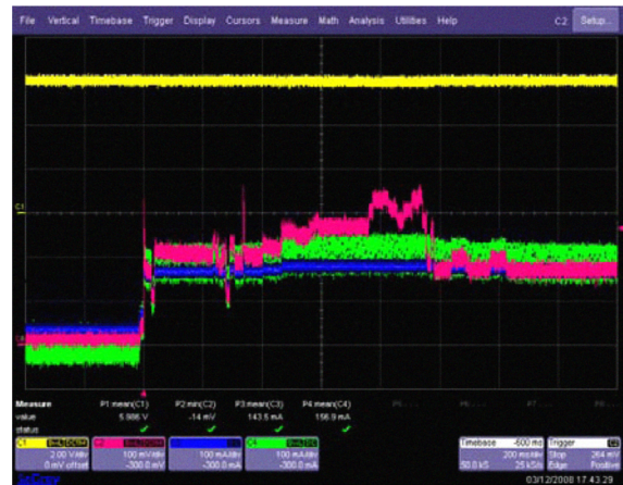
Fig. 5 .The inductor current (in green), the load current (in violet), the fuel cell current (in blue) and the output voltage (in yellow) under turning-on in playback mode.
