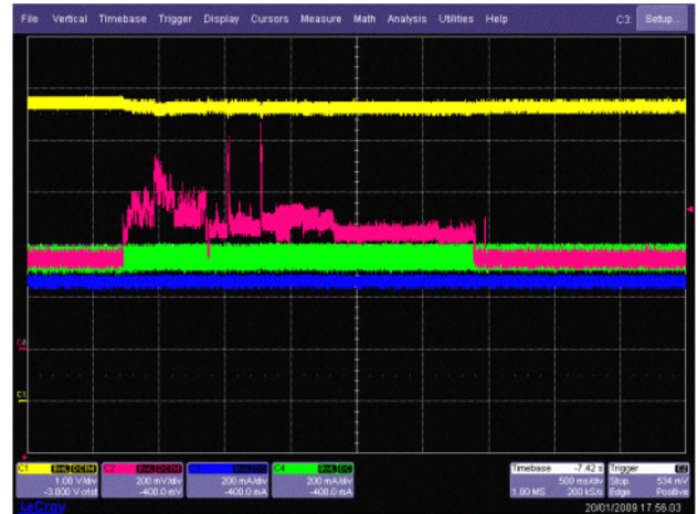
Fig. 4 .The inductor current (in green), the load current (in violet), the fuel cell current (in blue) and the output voltage (in yellow) under taking picture function.
