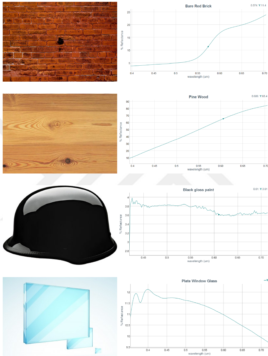
Figure 2.3. Spectral reflectances of reference materials in VL band [11].
