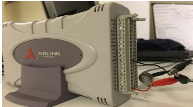
Figure 4.25. ADLINK USB-1902 device and input/output connections
