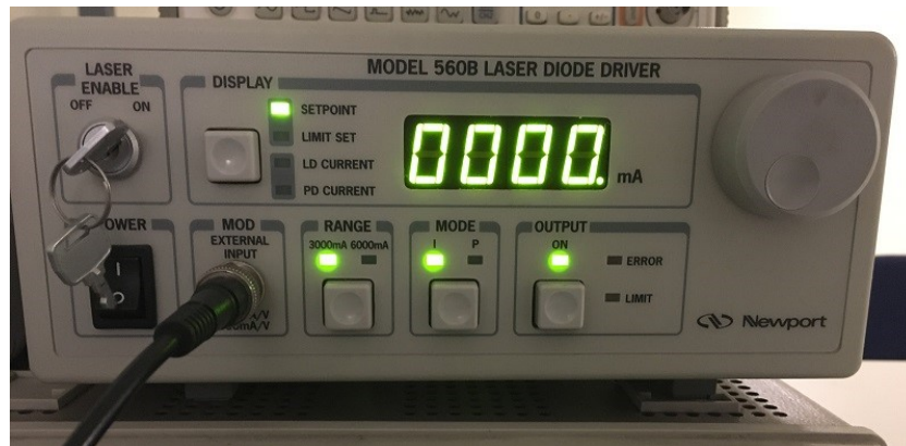
Figure 4.24. 560B Laser Diode Driver as a current source
