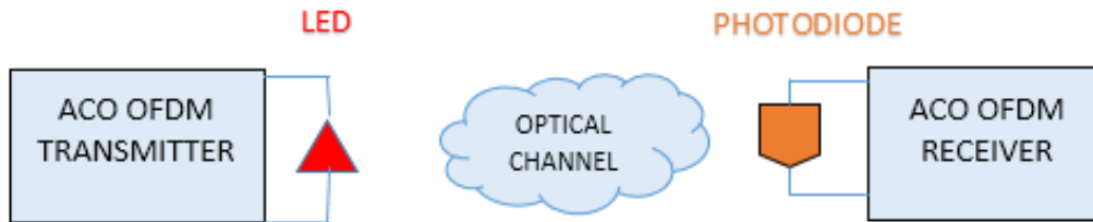
Figure 4.27. ACO OFDM Block Diagram for channel estimation
