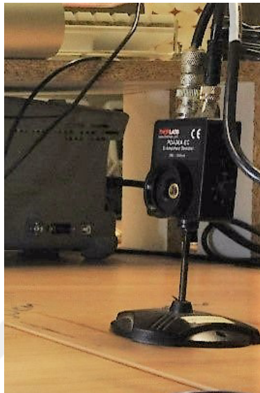
Figure 4.15. Receiver part of the 2nd generation PAM based VLC system
