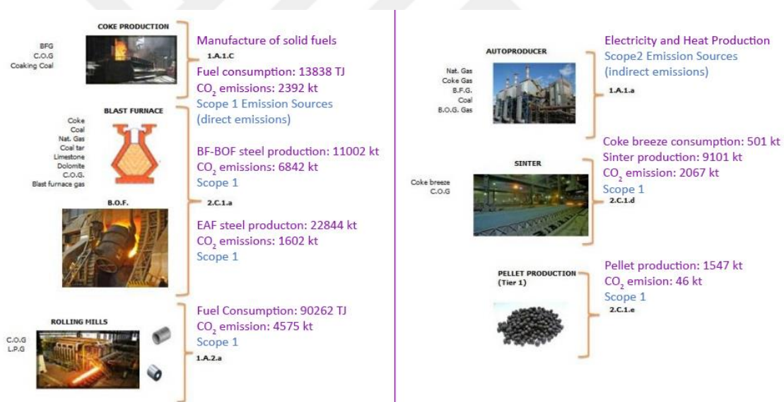
Figure 4.7 CO 2 emission sources of Turkish Iron and Steel Industry with the 2019-year consumption and CO 2 emissions data. (TurkStat, 2021a, 2021b).
